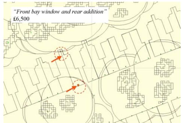
As can be seen from this brief extract, the root zone estimate – or “the zone where roots exist sufficient to cause ground movement resulting in damage a low rise building” – appears to be satisfactory.
